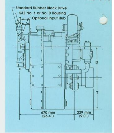
The MG-518-1 Marine Transmission is designed for the rugged service encountered by today's higher horse-power, harder working marine diesel engines.
